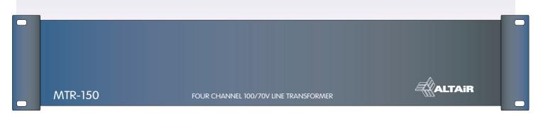
**MTR** 150/80 boxes are ideally suited as an accessory option for the Altair MA series multichannel amplifiers in 70 or 100 Volts P.A. line distributed audio applications. Each box contains four high quality, low LF distortion transformers. Special wound technics and high grade core materials ensures an extended low frequency operation down to 50 Hz at full power. Transient response is excellent, allowing the use in high performance music and speech applications.
