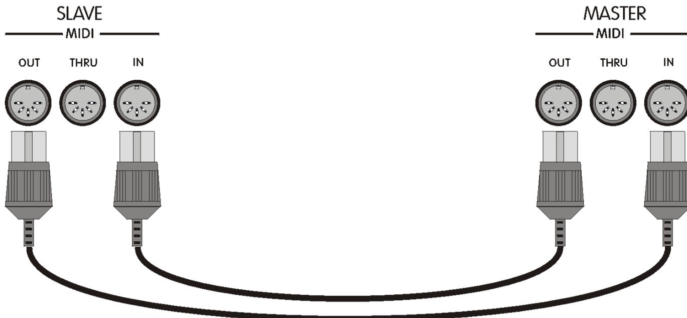
The reception and transmission MIDI channel must be the same in the MASTER unit and in the SLAVE one.
