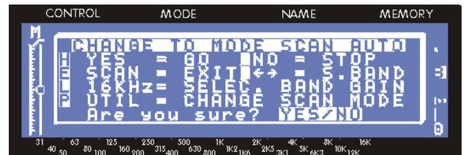
In the SCAN setup, you can equalise just as in the X/Y setup, but if a feedback is detected, its frequency will appear in the memory name place; you can therefore access the closest frequency and decrease the band value. You can also raise the channel volume up until the feedback appears and the equaliser indicates its frequency.
