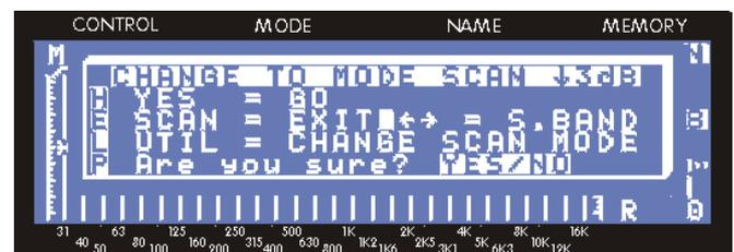
frequency, and the band corresponding to that frequency will decrease the selected decibels. If the feedback remains at the same frequency, press the YES key once again. In order to obtain a higher level, raise the volume again to the next feedback and continue this procedure.
